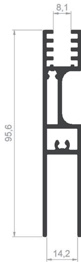
PROFILE CODE: 75422-00 WEIGHT: 1,310 Kg/m
