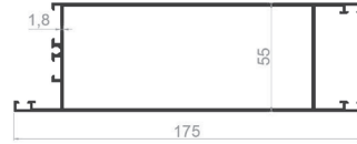
PROFILE CODE: 81010-00 WEIGHT: 2,282 Kg/m
