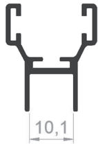
PROFILE CODE: 75458-00 WEIGHT: 0,236 Kg/m
