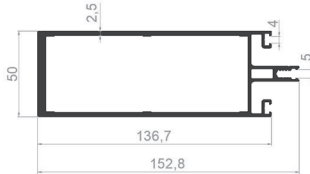
PROFILE CODE: 83016-00 WEIGHT: 3,143 Kg/m
